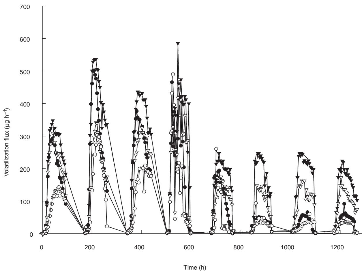
**Fig. 1** Volatilization flux ( $\mu\text{g h}^{-1}$ ) of 1,3-dichloropropene isomers from columns packed with the Arlington sandy loam, with and without organic amendment, after Telone-11 injection at 30 cm depth. Point differences indicate 4 h time intervals between sampling, and the data points indicated in the graph are for an 8-week sampling period. Cis = *Z* isomer and trans = *E* isomer. (●), cis; (○), trans; (■), C-cis; (□), C-trans
