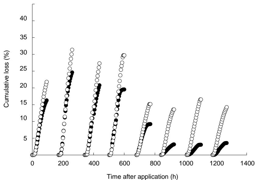
**Fig. 2** Cumulative volatilization losses in percentage of applied 1,3-D. (a) *Z* isomers from amended and unamended soils, and (b) *E* isomer from amended and unamended soils. (●), Amended soil, cis 1,3-D; (○), unamended soil, cis 1,3-D
