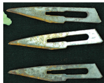
Figure 3: Corrosion caused by 1% HarvestCide® gel.
